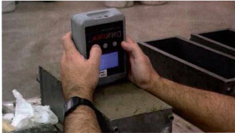
The Datatrace authenticator is being used here to detect tracing materials in concrete in the plastic state.
